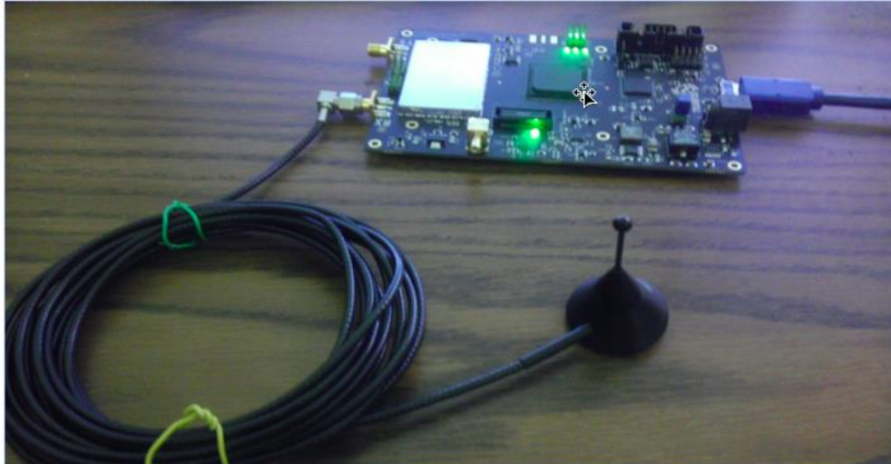
Figure 5. Nuand BladeRF with antenna to scan for I-Q values of raw signal.
